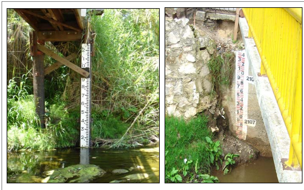
Picture 6.1. Gauging stations used to measure water flow on Carpinteria Creek in Santa Barbara (left) and in San Cristóbal (right).
