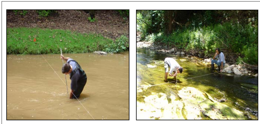
Picture 6.2. Measurements of the width and depths of a river cross section.
