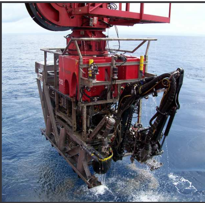
Figure 5. A Remotely Operated Vehicle (ROV) used to examine the active and inactive SMS deposits in Papua New Guinea
