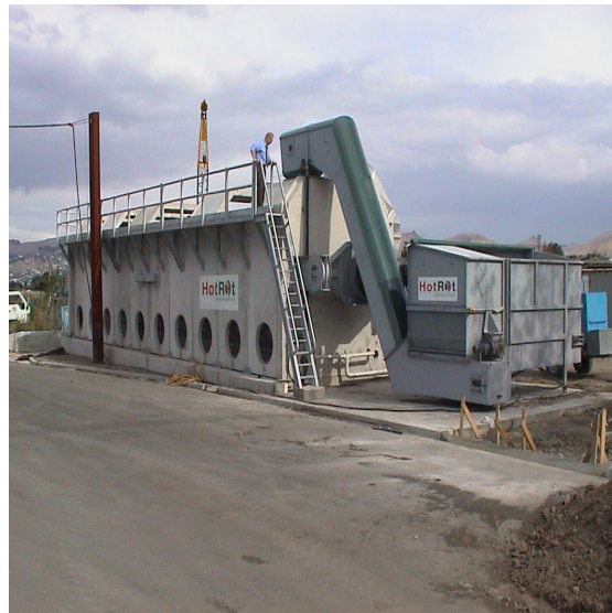
Figure 7-6: Hot-Rot in-vessel system.
