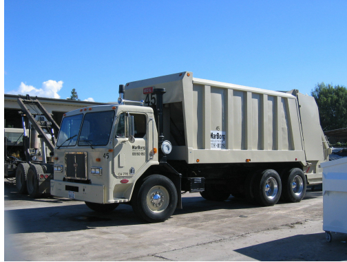
Figure 4-1: Marborg 11 ton front loader truck
