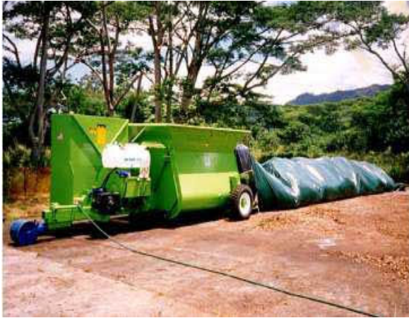
Figure 7-3: Picture showing an Ag-Bag system.
