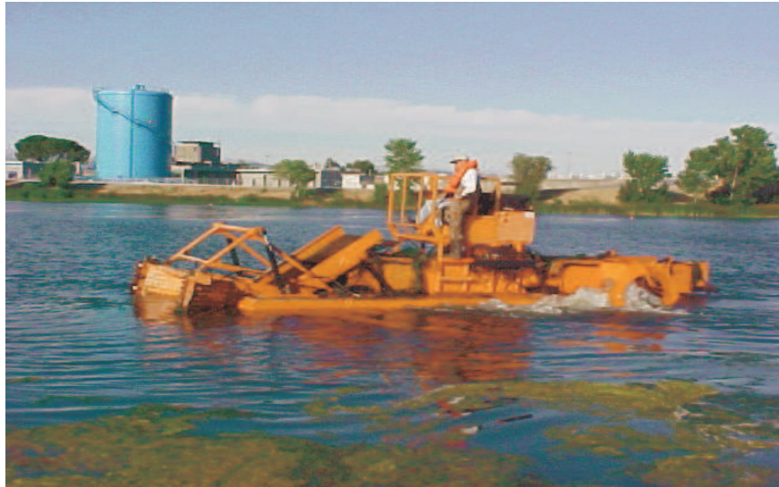
Figure 4. Mechanical harvester cutting an algae infestation. Photo: Dave Omoto, Solano Irrigation District.
