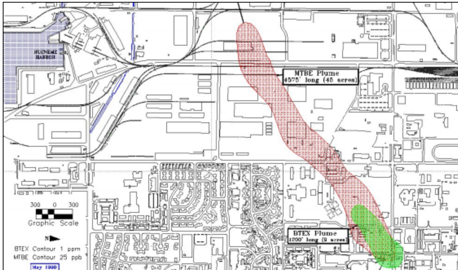
Figure 1. Graphical representation of areal extent of groundwater contamination as May 1999 at Port Hueneme Naval Facilities Engineering Service Center. Red area represents ~45-acre MTBE plume; green represents BTEX plume. (Source: NFESC)
