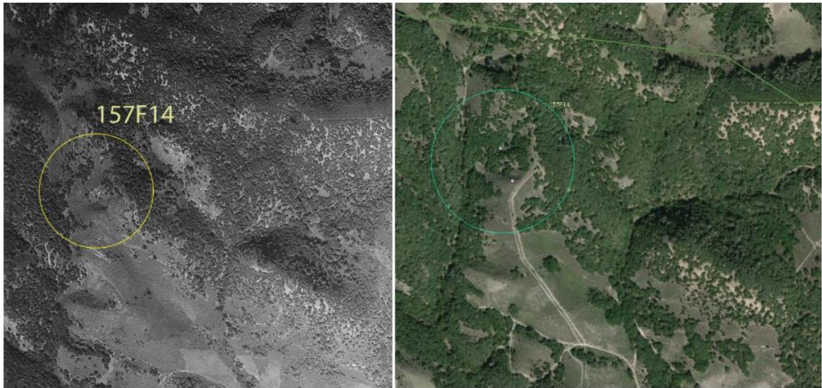
Figure A4-7. Aerial photographs and site topographic characteristic were used to relocate historical survey plots.
