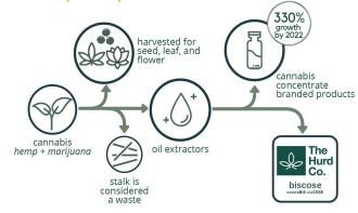
The Hurd Co collects waste from oil extractors, uses a low-impact pulping process to convert it into an apparel-grade MMC pulp, and sells it into the supply chain as
