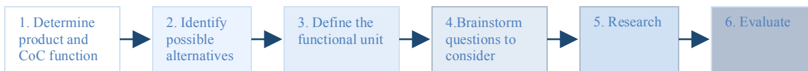
Figure A. Primary steps for incorporating life cycle screening into a First Stage Alternatives Analysis
