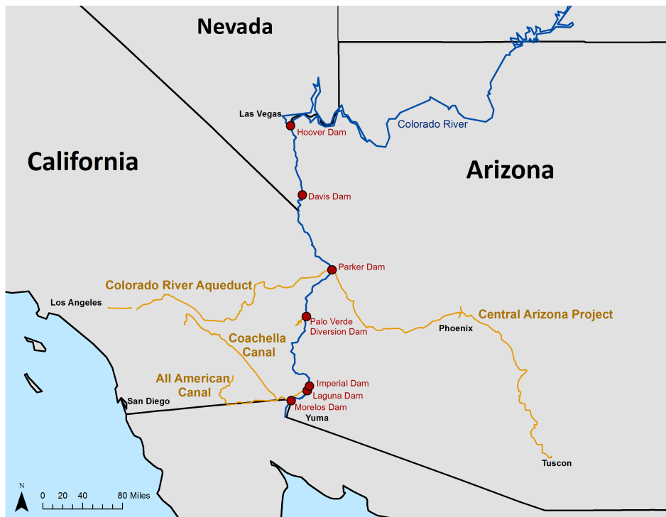
Figure 6: Water diversion infrastructure in the Lower Colorado River Basin. In California, the Colorado River Aqueduct diverts water for MWD, Palo Verde Irrigation District diverts water from Palo Verde Diversion Dam, the Coachella Canal delivers water to the Coachella Valley and the All American Canal delivers water to Imperial Irrigation District. In Arizona, the Central Arizona project diverts water from Lake Havasu, behind Parker Dam, to deliver water to the urban centers of Central Arizona. Finally, Nevada diverts water for the as Vegas area directly from Lake Mead, behind Hoover Dam.
