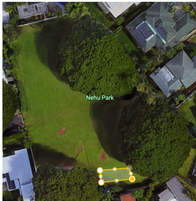
Figure 13. Theoretical placement of 900 ft 2 rain garden in Nehu Park, located in the Wailupe watershed. The rain garden is shaded yellow.
