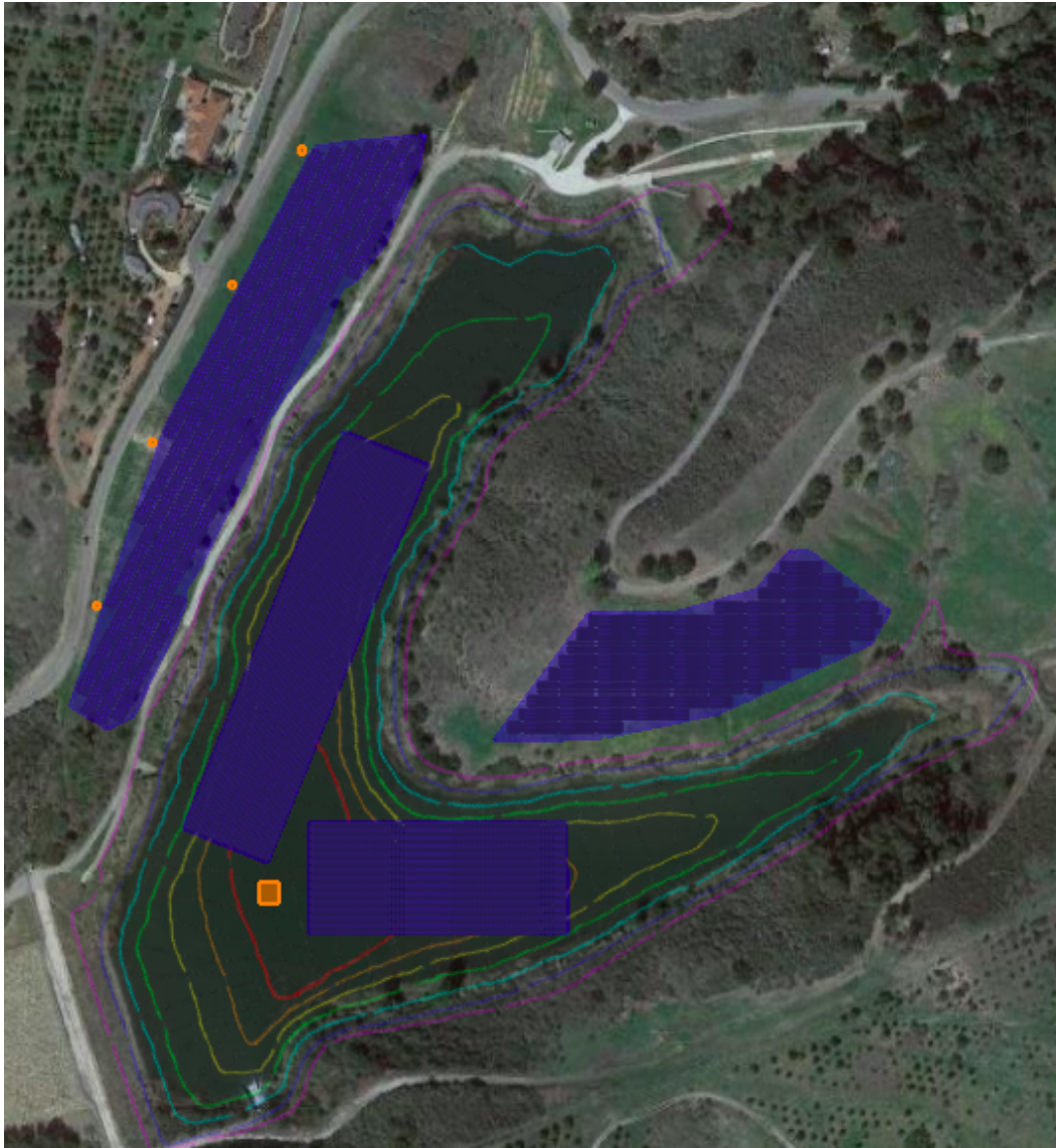
Figure 8. System design showing the full utilization of the site, with ground-mounted and floating systems. Blue represents array locations and orange represents a 'keepout buffer' around the intake tower and electricity poles. Represents the FOM5.7, FOM5.7 + BESS, and BTM5.7 systems.
