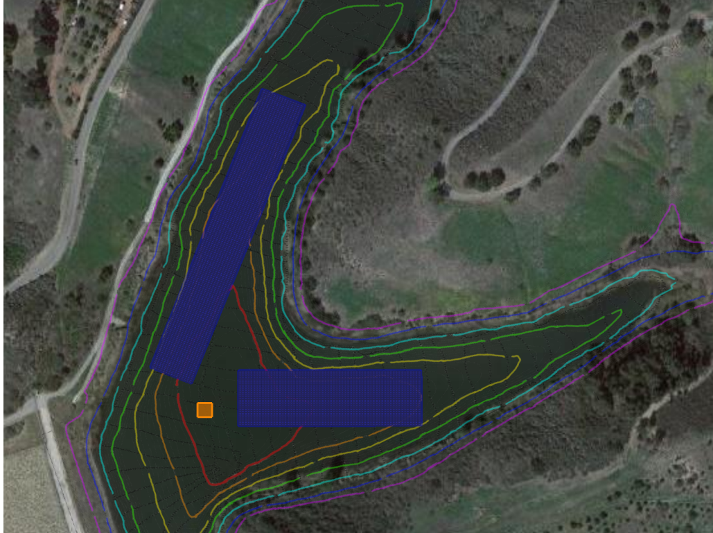
Figure 9. System design showing floating solar exactly sized to Cater’s load for a behind-the-meter system. Represents the BTM1.4 system.
