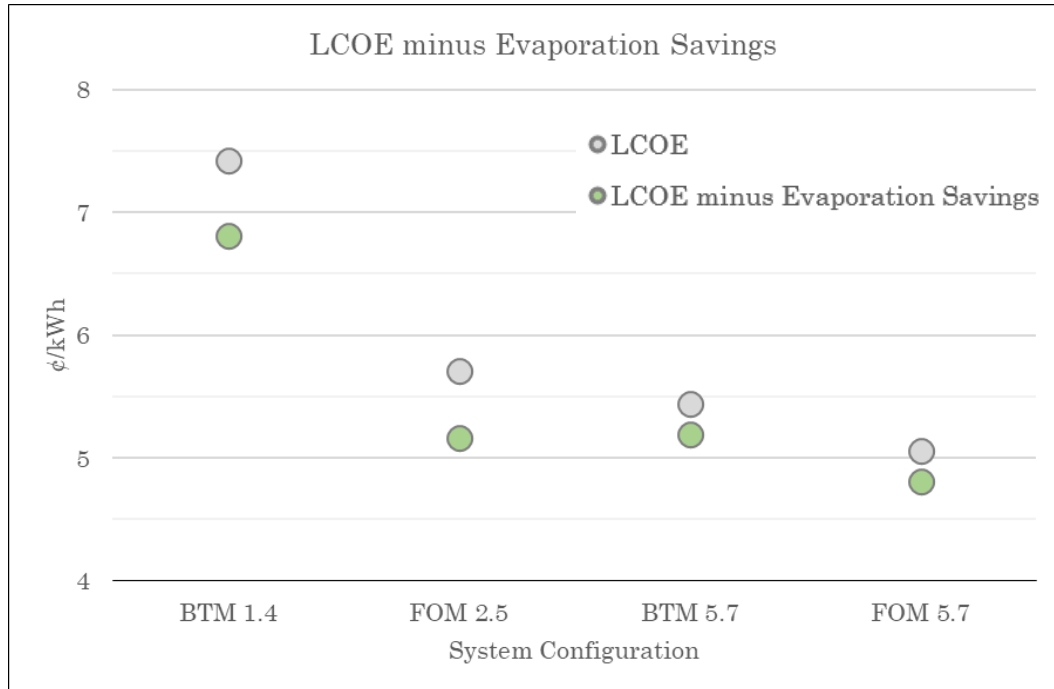
Figure 24. LCOE for each of the PV system configurations, excluding trenching or battery costs, adjusted for value added from reduced evaporation. Evaporation reduction values use the city of Santa Barbara’s water value and represent a 70% reduction in evaporation.
