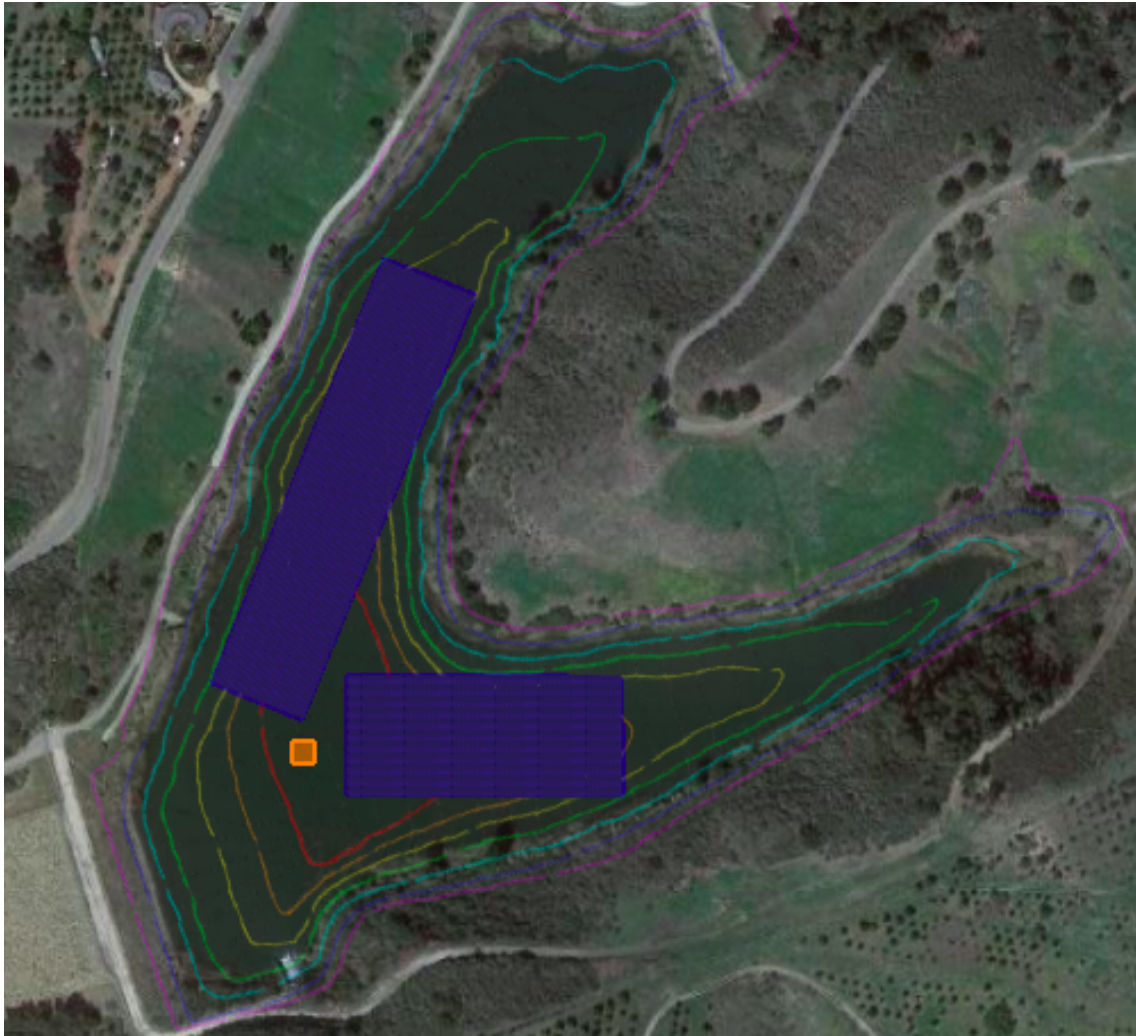
Figure 7. System design showing full utilization of the reservoir’s surface. Blue represents array locations and orange represents a ‘keepout buffer’ around the intake tower to be avoided. Represents the FOM2.5 system. Colored lines on the reservoir indicate the extent of the reservoir at various surface-level elevations.
