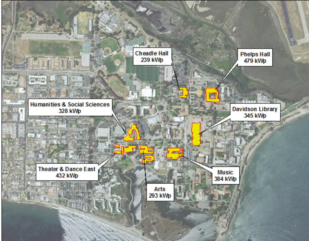
Figure 4: Second Priority Rooftop Recommendations. Estimated total capacity: 2.358 MW.
