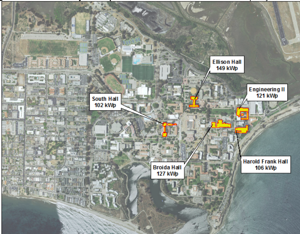
Figure 5: Third Priority Rooftop Recommendations. Estimated total capacity 0.812 MW.
