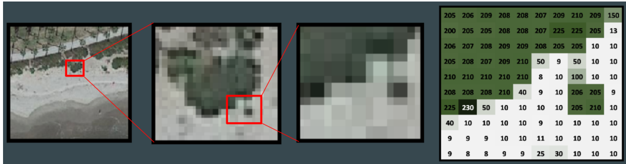
Figure 1. Visualization of a remotely sensed image that has been distilled into numbers, as is executed during the process of random convolutional featurization. This figure was produced for the purpose of scientific communication; it is not a true satellite image that has been distilled into features.
