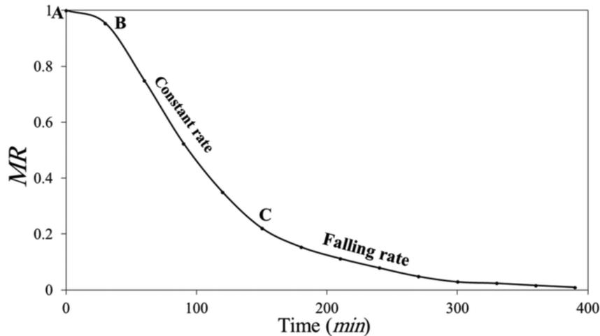
**Figure 27.** Drying curve of hot air drying at a temperature of 45 °C (Karimi et al., 2020)
