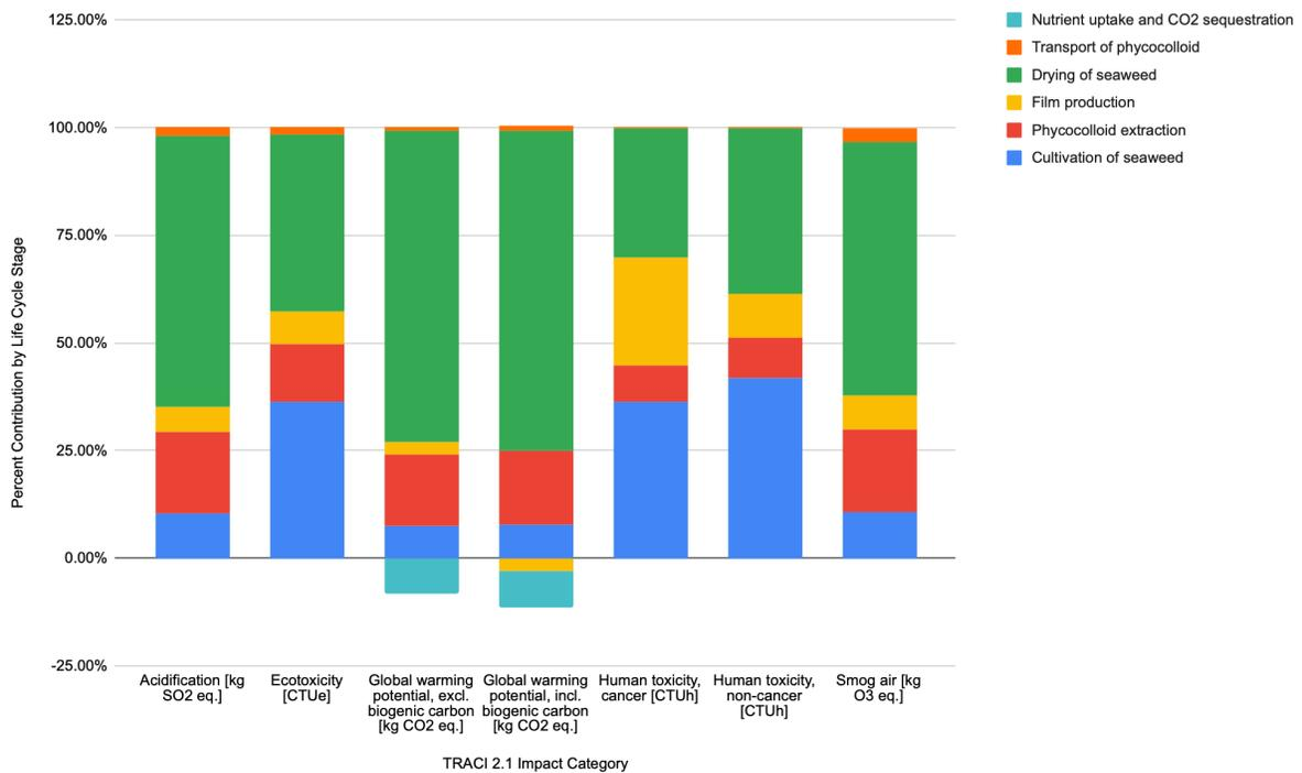
**Figure 5.** Contribution analysis of algal flexible film production scenario #1 for TRACI 2.1 impact categories. Refer to Figure 13 for impacts on eutrophication.
