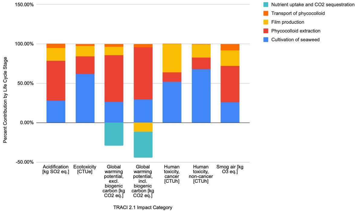
**Figure 7.** Contribution analysis of algal flexible film production Scenario #3 for TRACI 2.1 impact categories. Refer to Figure 13 for impacts on eutrophication.
