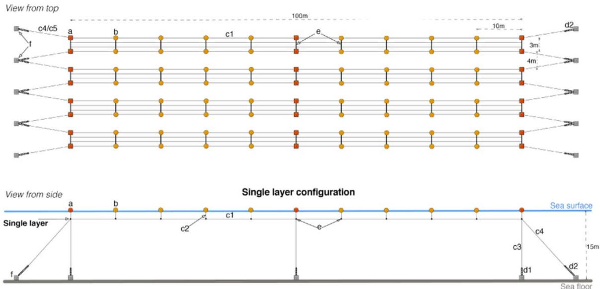
**Figure 3.** This figure was produced and published by van Oirschot et al. (2017). It shows a representation of longline cultivation infrastructure viewed from above and from the side, with components indicated according to the following: (a) marker buoys, (b) small buoys, (c) polypropylene rope (longline), (d) steel chain, (e) strip strengtheners, and (f) concrete anchors.
