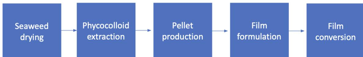
**Figure 4.** System diagram for seaweed processing from seaweed drying to film conversion.
