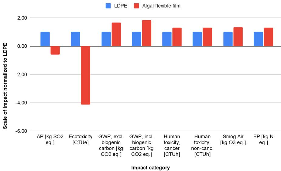
**Figure 22.** End-of-life impacts for LDPE and algal flexible film, with LDPE normalized to 1.
