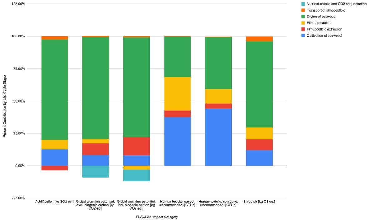
**Figure 9.** Contribution analysis of algal flexible film production Scenario #5 for TRACI 2.1 impact categories. Refer to Figure 12 for impacts on ecotoxicity and Figure 13 for impacts on eutrophication.
