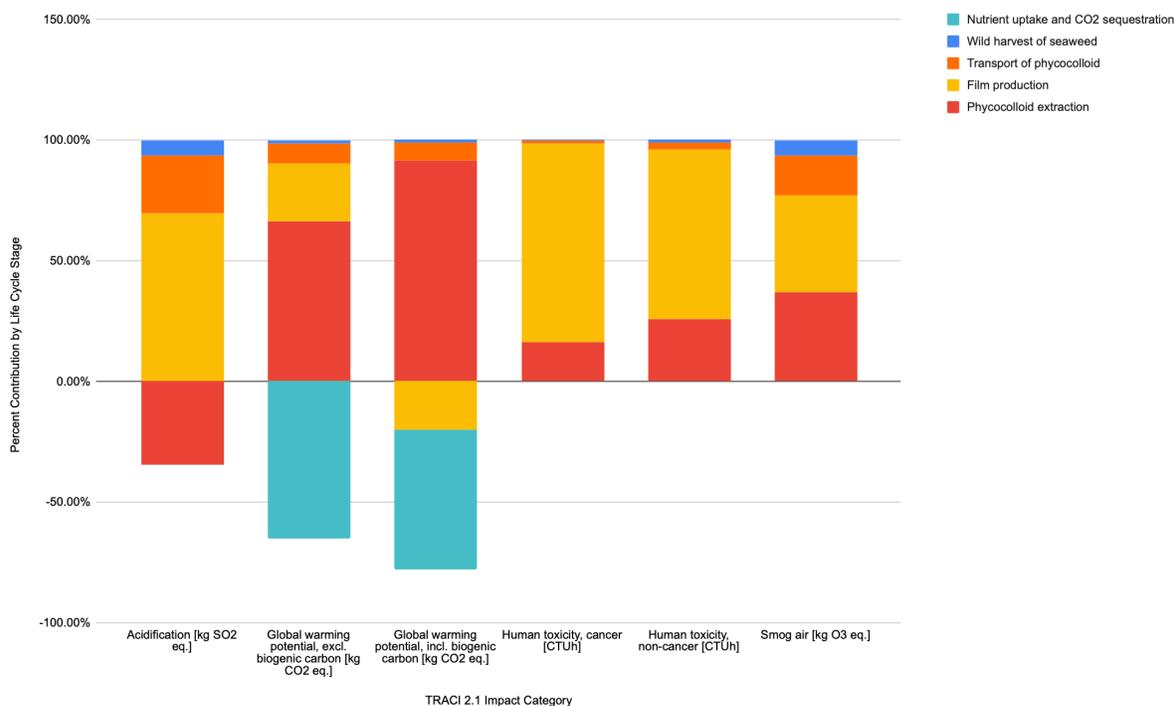
**Figure 10.** Contribution analysis of algal film production Scenario #6 for TRACI 2.1 impact categories. Refer to Figure 12 for impacts on ecotoxicity and Figure 13 for impacts on eutrophication.
