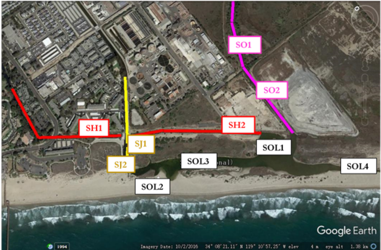
Figure 8.12. Distribution of sampling points at Ormond Lagoon. Label: SH (Hueneme Drain) in red; SJ (J-Street Drain) in yellow; SO (Oxnard Industrial Drain); SOL (Sampling points in Ormond Lagoon) in black. SOL points are sorted by near the Superfund Site (SOL 1) or not (SOL 2-4). SOL 4 is away from all three main drainages.
