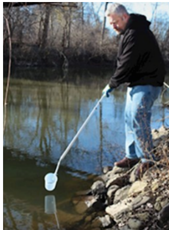
Figure 8.16. Field sampling with a water sampling dipper.
