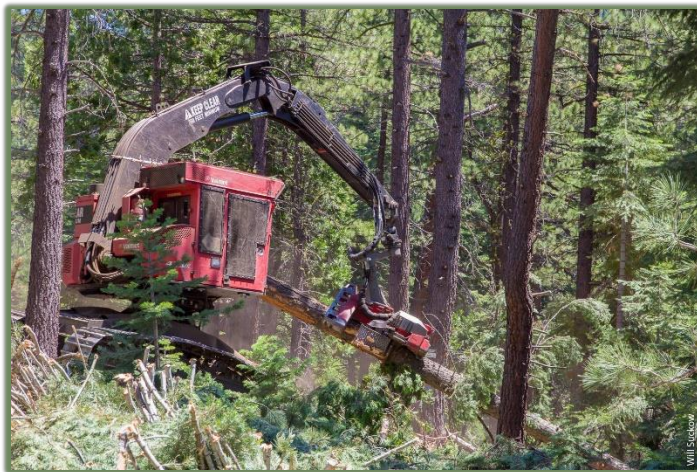
Figure 3-8. Mechanical treatment by feller-buncher (photo credit: USFS Yeti Fuels Reduction Project).
