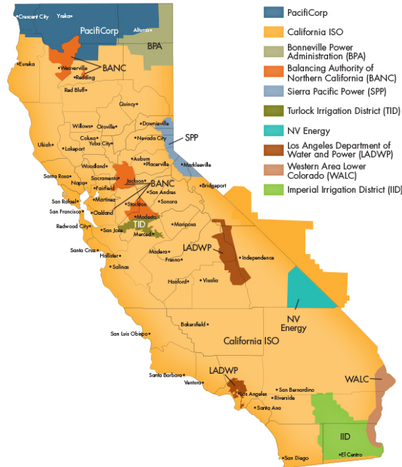
Figure 1. CAISO’s operational territory covers 80 percent of California and a small portion of Nevada, including the service territories of California investor owned utilities and the service territories of some municipal utilities. There are a few small areas within CAISO where the local power companies manage their own transmission systems.
