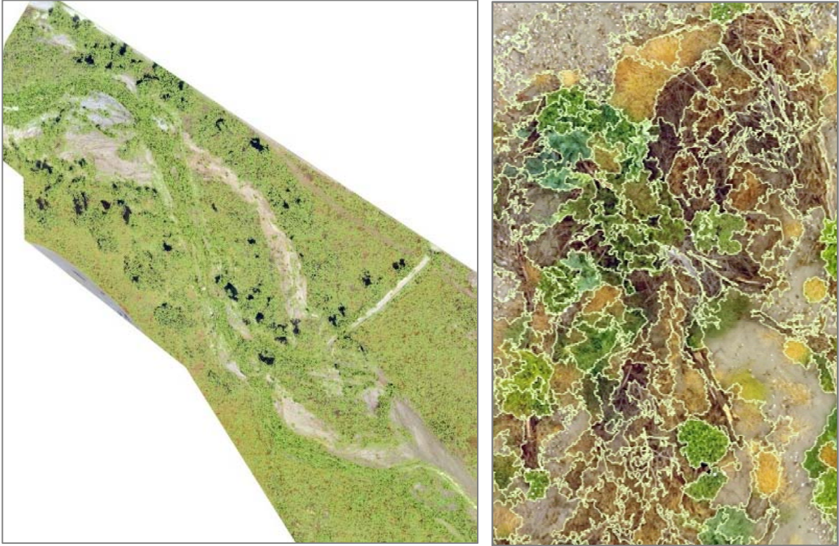
Figure 11. LEFT: segmentation layer of the full region of interest in the northeast section of Panofsky Field; RIGHT: A close-up of the segmented polygons layer overlaid on top the DJI Phantom 4 imagery.
