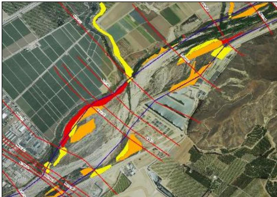
**Figure 7.** Example of HEC-RAS cross section geometry modification. HEC-RAS cross sections (red lines), were imported into ArcGIS and overlaid on polygons of *A. donax* density (yellow, orange, and red polygons). HEC-RAS cross sections Manning's  $n$  coefficients were then modified to reflect the amount of intersection with *A. donax*.
