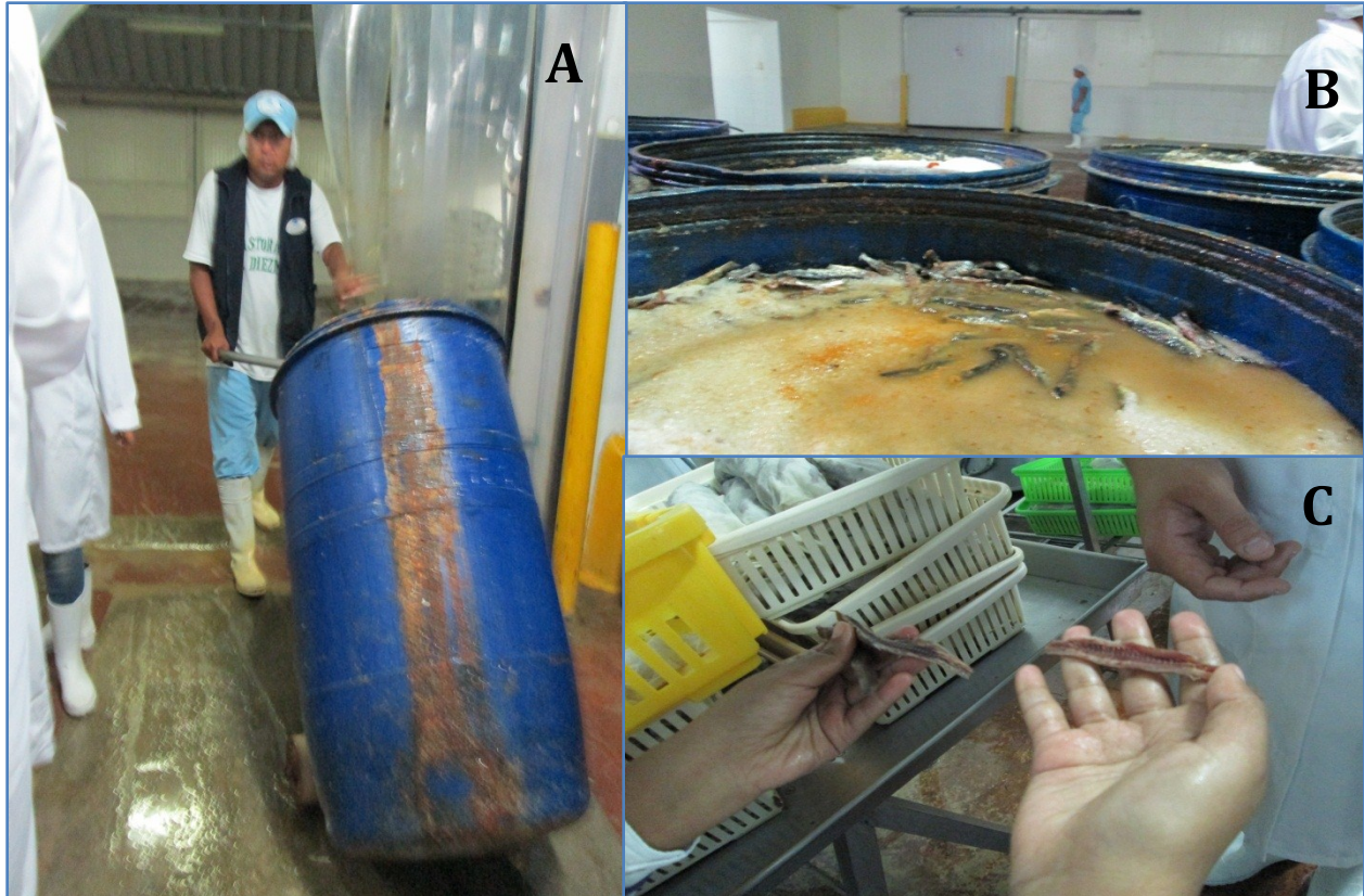
Image 2: Anchoveta fillets are salted and cured in barrels for 6 months or more (A, B). The final fillets are then cleaned (C) and packed into aluminum cans for export. Photo credit: Yoel Kirschner (July 2012; Compania Americana de Conservas Pisco, Peru ).
