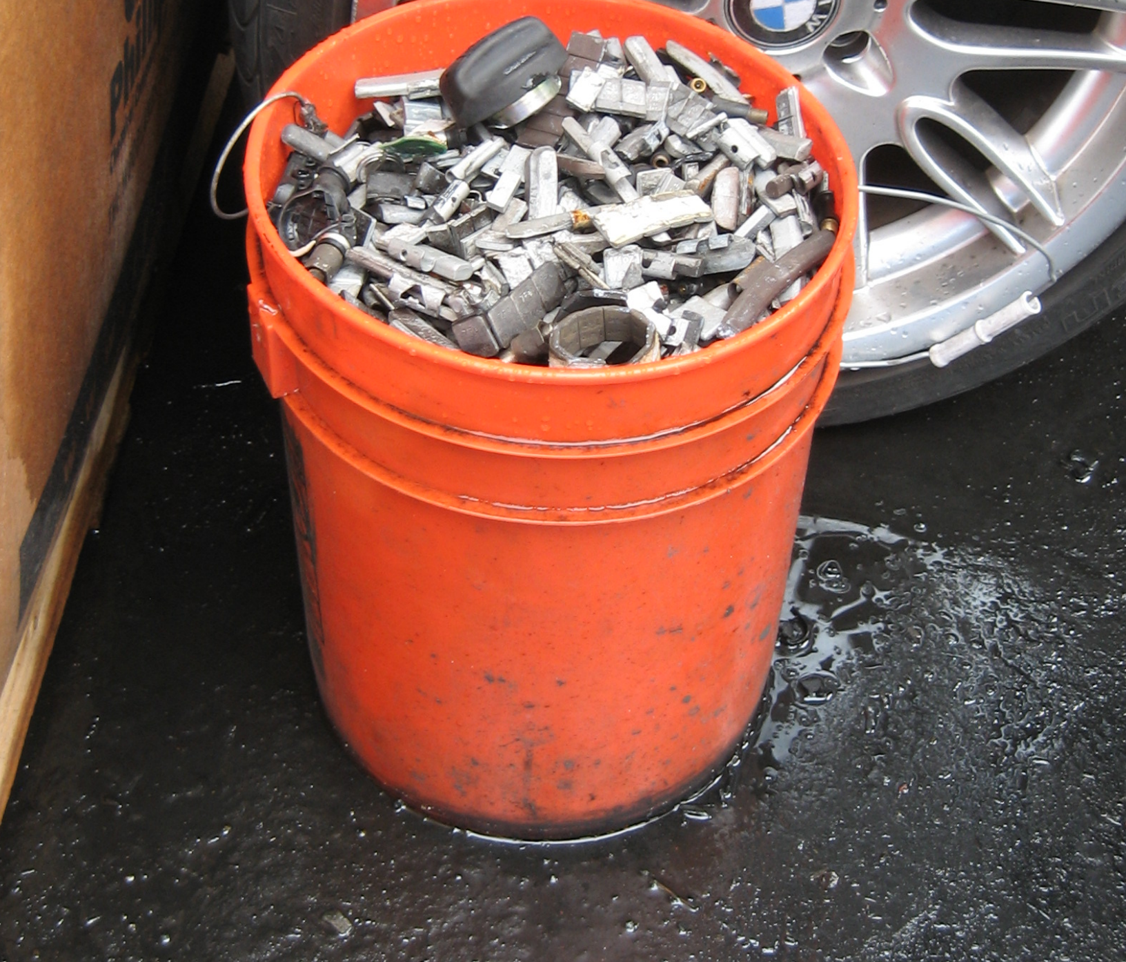
Figure 9: Lead wheel weights recovered by the dismantler. Photograph taken at LKQ Corporation facility.
