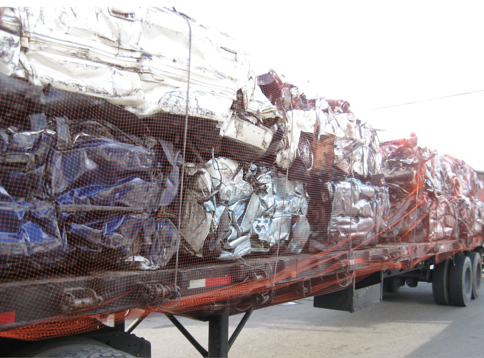
Figure 6: Crushed hulks being delivered to a shredding facility. Photograph taken at SA Recycling facility.
