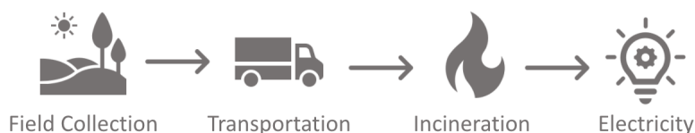
Figure 7. Incineration process diagram. After field collection and transportation, APW is mixed with MSW and combusted. The resulting heat is collected and converted to electricity.
