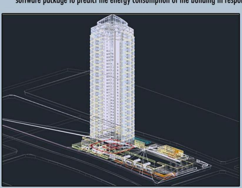
Our models show that increasing exterior-wall insulation beyond R-13 in a building with an 80% glass façade has an insignificant effect on reducing heating and cooling loads in San Francisco's mild climate. For windows, our models show that low solar heat gain is the most important factor in reducing annual energy consumption for the proposed building.
