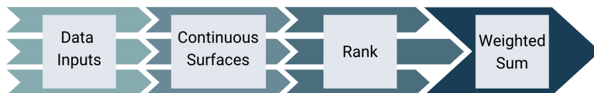
Figure 3.1 Workflow used for data analysis in the decision support tool. Data inputs were interpolated to form continuous surfaces for the project study area. Values were then ranked and classified according to relative recharge suitability before being combined through a weighted sum. The workflow was repeated to provide outputs for suitable recharge locations, surficial nitrogen balances, and additional considerations.
