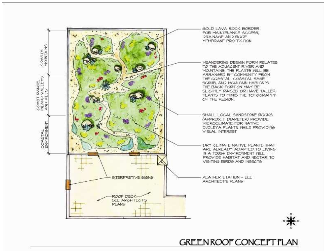
Figure W4: Green Roof Drawing for the Limoneira Company [Courtesy of the Limoneira Company]
