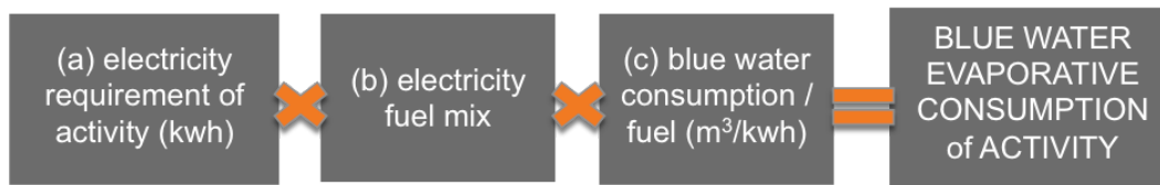
Figure 9: Method used to convert electricity requirements to water consumption.
