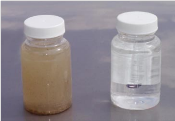
Figure 14a. Septic tank (left) versus wetland (right) effluent.
