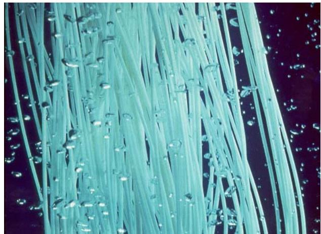
Figure 2. Hollow-fiber membranes (Image from GE/Zenon)
