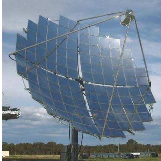
Figure 30. Solar Systems 20 kW CPV dish (NREL, 2007c).
