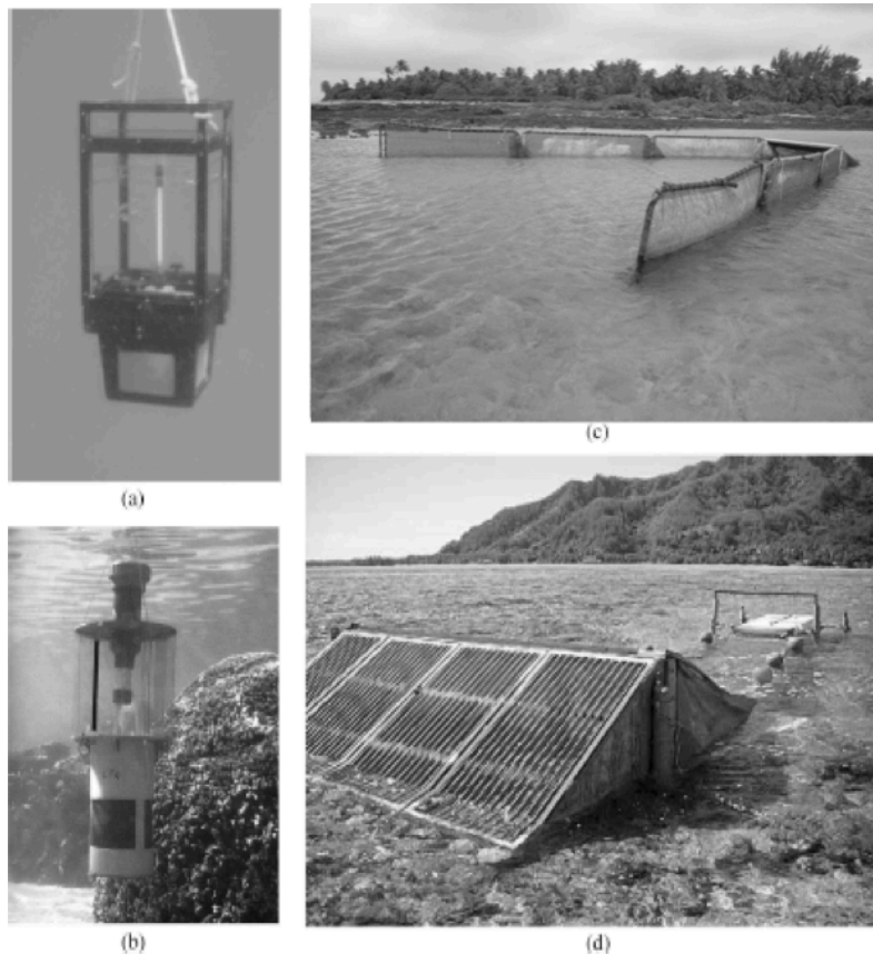
Figure 11. Examples of post-larval capture devices (a,b) Light traps, (c) hoa net, and (d) crest net. Adapted from Bell et al. (2009).
