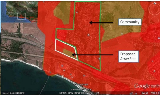
Figure 2 SCE Interconnection Map - Red suggests poor siting with increased interconnect costs likely
