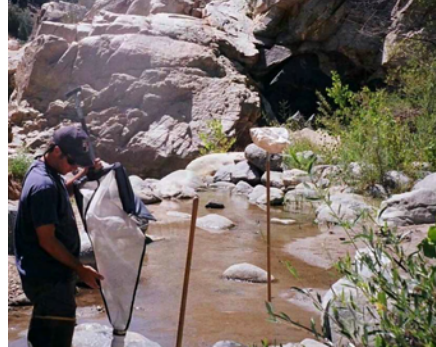
Figure 4. Ben Livsey collecting a macroinvertebrate sample with a 0.5mm mesh Surber sampler.
