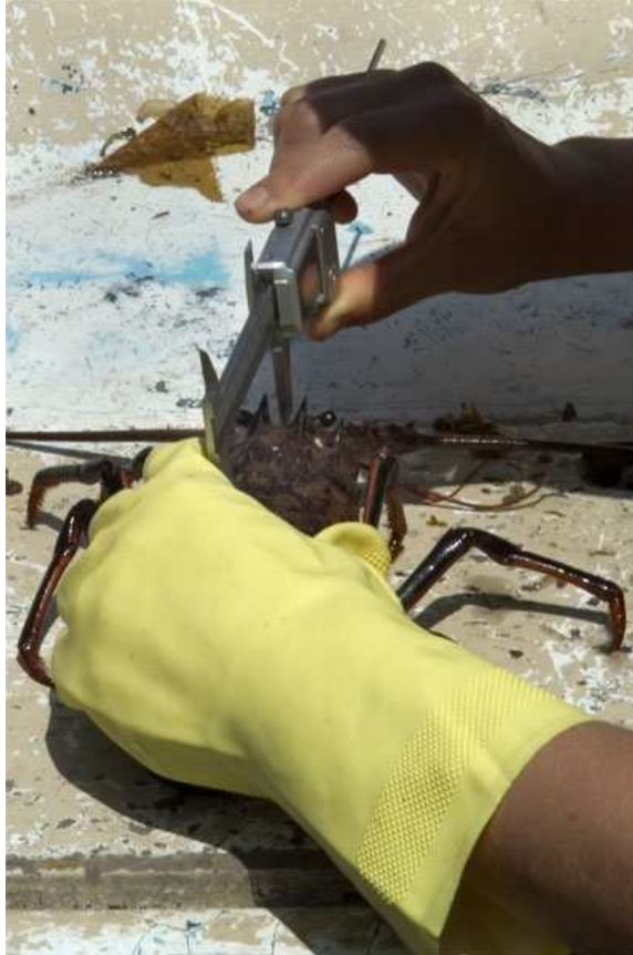
Figure 28: Carapace Length. In this photo, a Bren researcher is measuring the carapace length of a lobster with vernier calipers.
