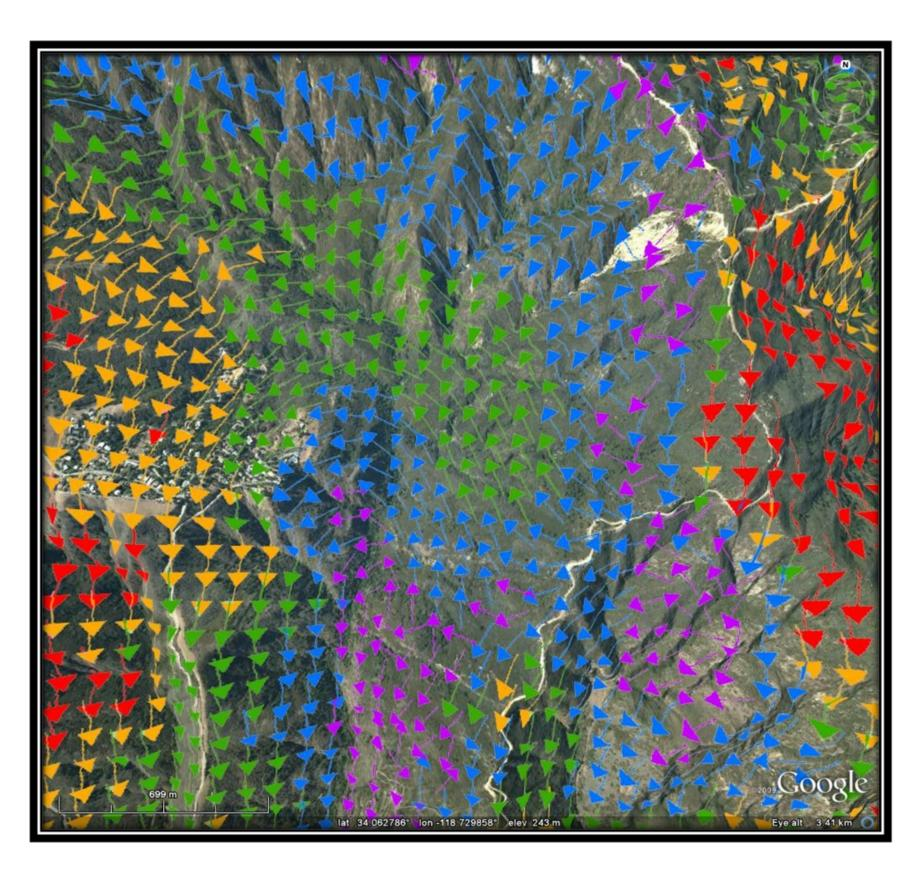
A 90 degree, 15 mph surface wind layer for Corral Canyon (shown in Google Earth) illustrates the effect of topography on wind speed and direction (shown by colored arrows). Red indicates high wind speeds, and fire simulations in this study. purple low wind speeds.
