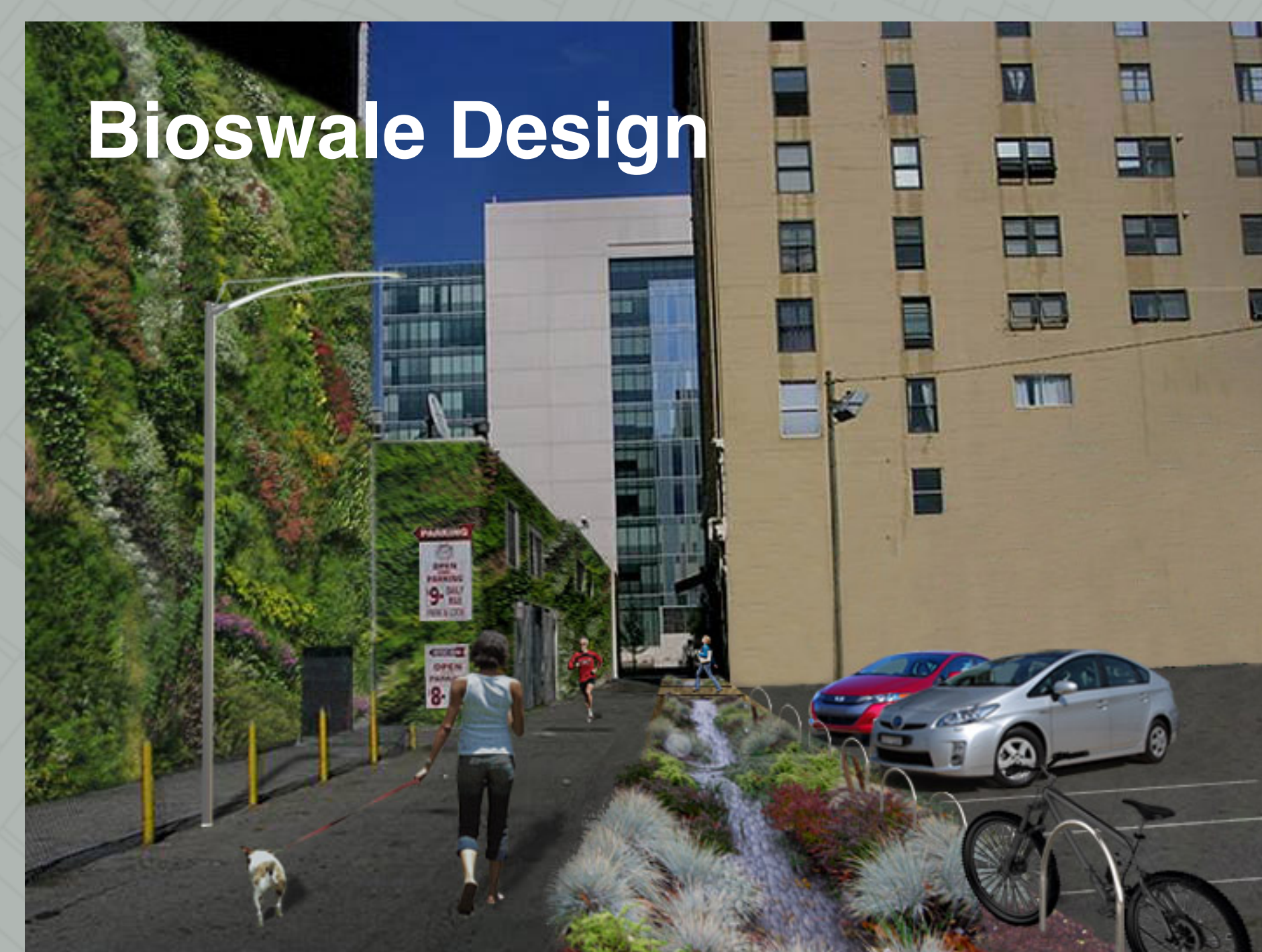
Bioswale Design •improves microclimate •captures all site stormwater & >50% of drainage from building rooftops
