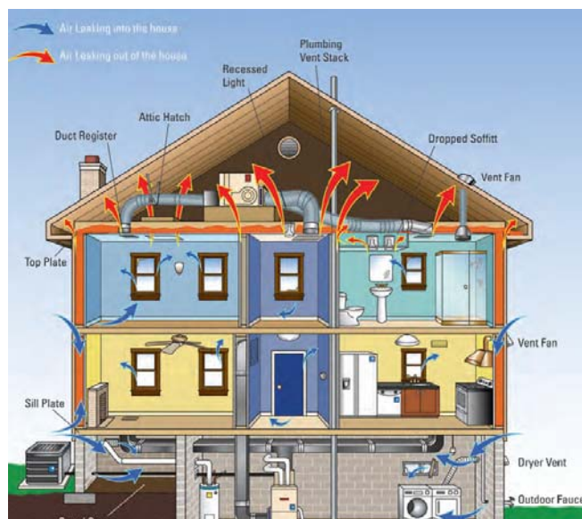
Figure 11: Leaks in the building envelope allow outside air to enter the home and conditioned air to leave the home, resulting in lower comfort and higher utility expenses.
