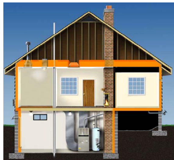
Figure 12: Insulation helps keep your house warm in the winter and cool in the summer by preventing the free flow of air between your house and outdoors.
