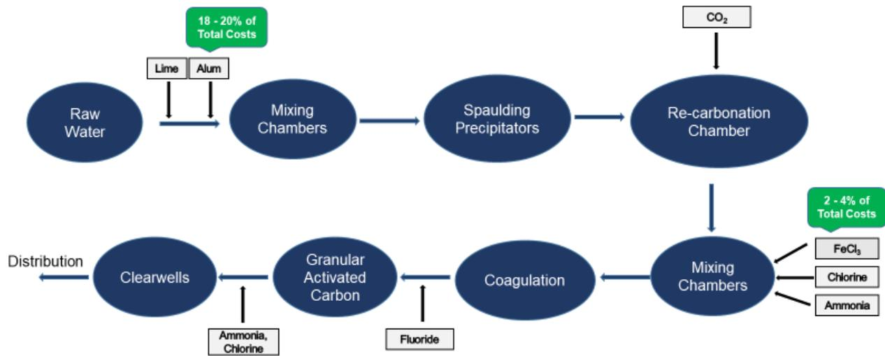
Figure A1. Schematic of the drinking water treatment process at Minneapolis.
