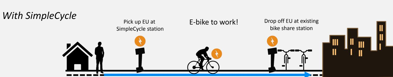
To incorporate electric power into existing bike share systems, new peripheral stations provide cyclists beyond the coverage area of the existing bike share with access to electric power for their personal bikes, and leverage the existing network as pick-up and drop-off locations for the electrification units (EUs). Additionally, the electrification units can be used within the city on bike share bikes.
