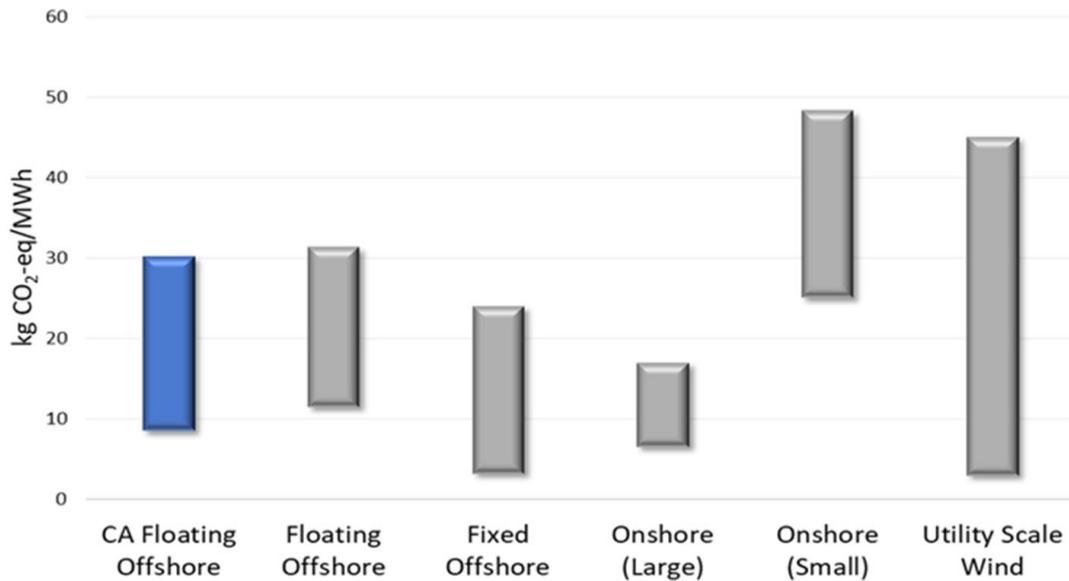
Figure 22. Comparison with previous wind energy LCA results.
