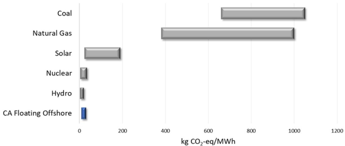
Figure 23. Comparison of GHG emissions from floating offshore wind and other energy sources.<sup>83</sup>
