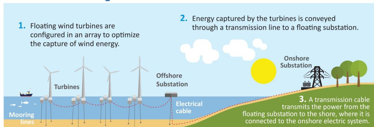
Figure 2. A general overview of a floating offshore wind farm. The wind turbines are connected to the ocean floor with mooring lines and an anchoring system. Then electric array cables connect the turbines to an offshore substation which then transmits the energy to the onshore grid.<sup>5</sup>
