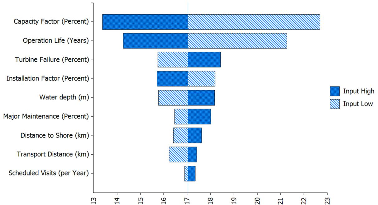
Figure 21. Total GWP (kg CO<sub>2</sub>/MWh) tornado diagram showing the largest contributors to the variability in GWP results. The dark shading shows what happens at the high end of each parameter. For example, the higher the Capacity Factor, the less emissions per MWh, but the higher the transport distance the more emissions per MWh.
