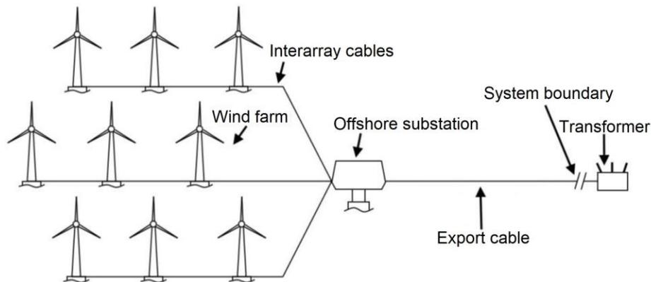
Figure 7. System boundary for a representative floating offshore wind project, adapted from Thomson and Harrison, 2015.<sup>28</sup>
